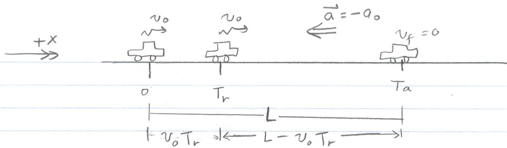
(b). The Eq's in Table 2.2 are valid only if  $a = \text{const.}$ . So we can apply them separately in time intervals  $0 - T_r$ , and  $T_r - T_a$ .
