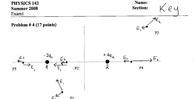
The figure shows two charges located at the positions shown. Calling the electric field due to the -3q charge as  $E_1$  the +4q charge as  $E_2$ , answer the following questions.
