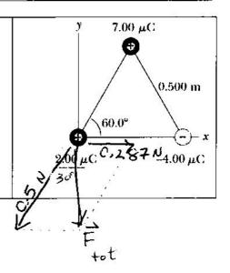
$\frac{7\mu C}{\Theta}$   $0.5m = \frac{7\mu C \times 5\mu C}{(0.5m)^2} = 0.5 \text{ Newton.}$
