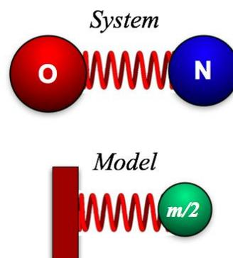
Some consideration of the Newton’s law equations for masses and springs shows that the oscillation of a system consisting of two masses of mass  $m$  connected by a spring with spring constant  $k$  is described the same equation as a single mass with mass  $m/2$  connected by a spring with spring constant  $k$ . So we can use this system (with  $m \sim 15$  Daltons) as a model of our diatomic vibrations.
