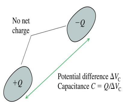
Consequently, the capacitance depends only on the geometry of the electrodes.
