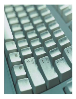
The keys on most computer keyboards are capacitor switches. Pressing the key pushes two capacitor plates closer together, increasing their capacitance.
