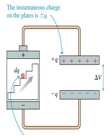
The charge escalator does work  $dq \Delta V$  to move charge dq from the negative plate to the positive plate.
