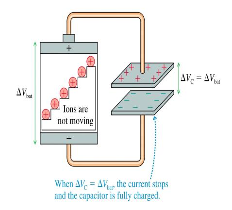
Capacitance always refers to the charge per voltage on a fully charged capacitor. • The ratio of the charge Q to the potential difference  $\Delta V_C$  is called the **capacitance** C:
