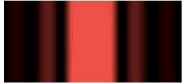
Diffraction from one (wider) slit
