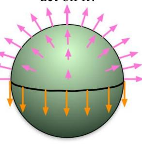
$F_{\text{air pressure inside} \to \text{top half}}^{\uparrow} = \frac{1}{2} pA = \frac{1}{2} p(2\pi r^2) = \pi pr^2$
