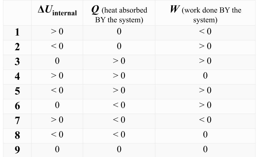
An inflated balloon is place in a vacuum chamber and some of the air removed. The balloon grows substantially in size. What happened to the energies of the air inside the balloon?
