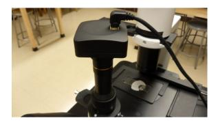
Camera can be rotated using the adjustable pin below the lens.
