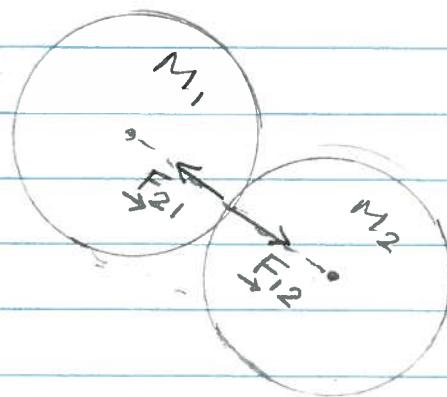
occur, if there is no external force the internal forces always come in action-reaction pairs and therefore the total vector momentum  $\vec{P}$  of the system cannot change.
