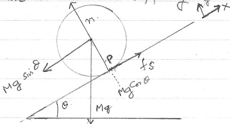
Now it will have both a linear acceleration and an angular acceleration.
