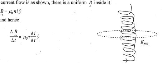
The problem has cylindrical symmetry about axis of solenoid,  $E_{\it NC}$  at r must be a function of r only and must be azimuthal. Let i increase with time. Then flux of B along  $+\hat{y}$  is increasing with time. Take a circular loop. As shown direction of  $E_{NC}$  must be clockwise ( as viewed from above) to oppose increase of  $\Phi_B$ .
