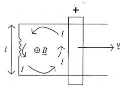
and Lenz's Law tells us that the induced  $\varepsilon mf$  must oppose the increase in flux of  $\underline{B}$  into the page requiring negative at the bottom and plus at the top leading to a counterclockwise current.
