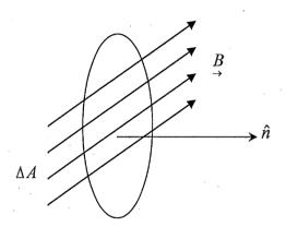
is along  $\hat{n}$ . Then, as in the case of E, we define flux of B through  $\Delta A$  to be
