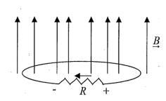
and the direction of  $E_{\it NC}$  in the loop must be clockwise. Current in  $\it R$  will flow from left from right.
