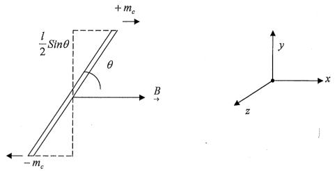
And we find that it experiences a Torque:  $\underline{\tau} = -m_c lB \sin \Theta \hat{z}$  or  $\underline{\tau} = \begin{bmatrix} \mu \times B \\ \rightarrow \end{bmatrix}$  with  $\mu = m_c l$
