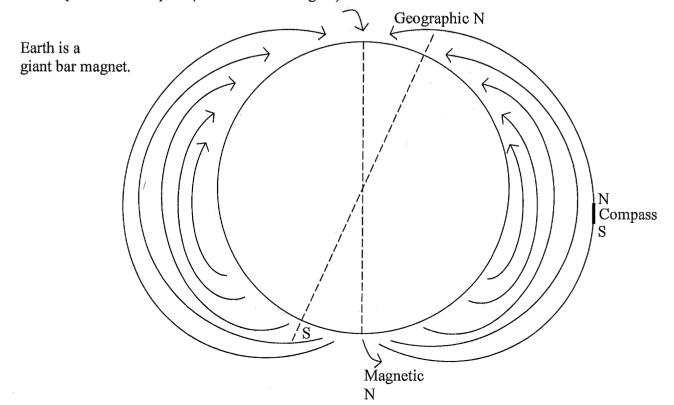
To understand this let us pretend that the B.M. can be imagined as consisting of magnetic "charges"  $\pm m_c$  separated by l.
