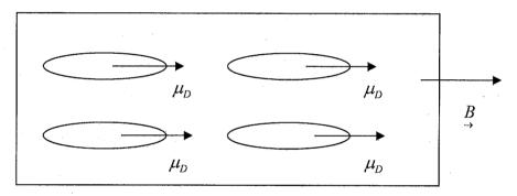
and every domain has its  $\mu_D$  along direction where it prefers to stay. So next if we remove B, the  $\mu_D$ 's will stay put, the Bar has a "permanent" magnetic moment. Indeed, we have "constructed" a
