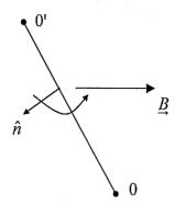
And the torque will turn  $\hat{n}$  toward  $\underline{B}$ , counter clockwise so for a dc motor we established a current in a coil, suspended in a  $\underline{B}$  field, and free to rotate about an axis perpendicular to  $\underline{B}$ , and reverse the current every half cycle using a commutator and brushes.
