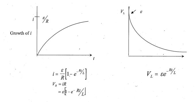
After this long time  $i = \frac{\varepsilon}{R}$  and a magnetic field has been established in L and stores  $\frac{B^2}{2\mu_0}$  of energy per  $m^3$ . So now if we move the switch so  $1 \rightarrow 3$  the circuit becomes
