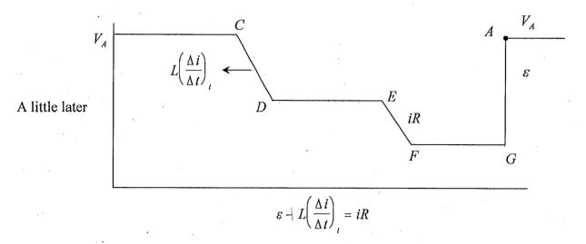
Clearly,  $\left(\frac{\Delta i}{\Delta t}\right)_t < \left(\frac{\Delta i}{\Delta t}\right)_0$  Rate of growth has slowed down.
