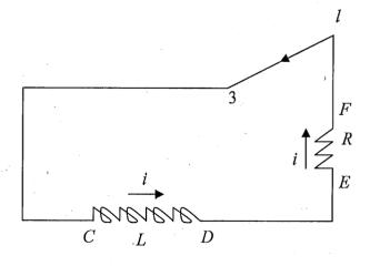
No Battery in circuit. Magnetic Energy stored in L is source of current!
