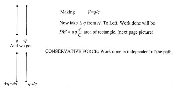
To build up charge from 0 to Q you need area of  $\Delta$ . This work is now  $U_E = \frac{1}{2} \cdot Q(Q/C) = \frac{Q^2}{2C}$
