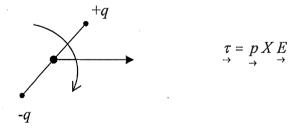
Every dipole feels a torque which makes it parallel to the E-field between the plates hence the system looks like what is shown on the next page:
