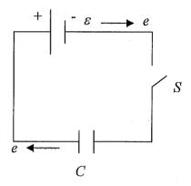
Note: the lines connecting the devices are perfect conductors and so under stationary conditions they must become equipotentials. That is if we close the switch S and wait for a while the Potential difference across C will become  $\varepsilon$ .
