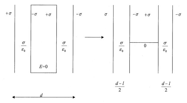
That is, as if two capacitors were in series, Each having  $C_1 = C_2 = \frac{2\varepsilon_0 A}{d-l}$  (2)
