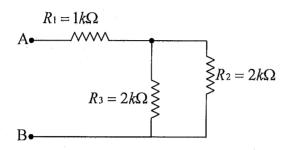
$R_2$  and  $R_3$  are in parallel so
