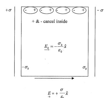
Dipole in E -field experiences torque, which causes each Dipole to line up along E.
