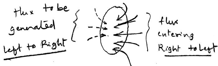
But, by the right hand rule, the current has to be as shown below to produce a flux from Left to Right.
