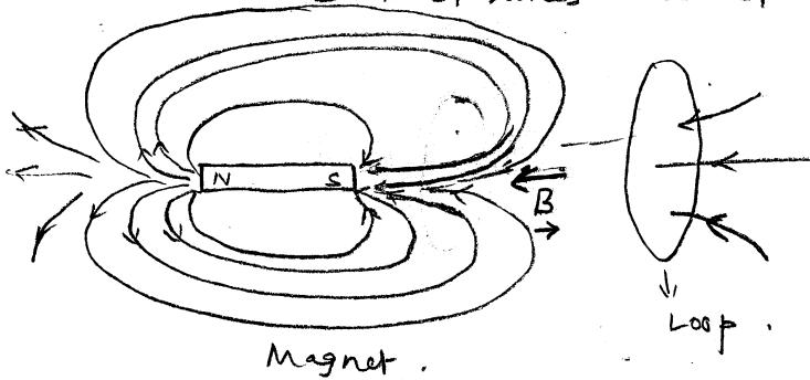
As shown in the figure, the flux through the loop is in the direction opposite to the direction of motion of the magnet increases, as the south pole approaches the loop. This is because magnetic field lines start at the North pole and end on the South pole.
