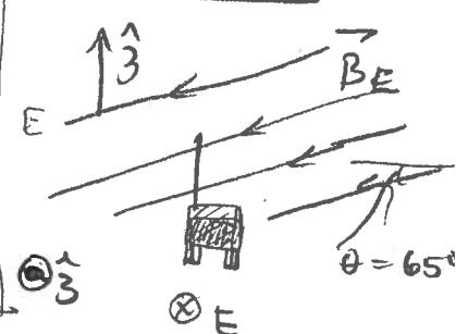
The car should travel East to maximize induced voltage in the desired way.
