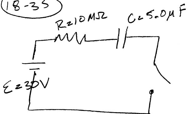
$q(t) = Q_{\max} (1 - e^{-t/\tau}) \rightarrow$  charge on the capacitor as a function of time.
