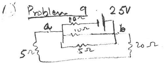
$$\begin{aligned} \text{a) } R_{eq} &= 20 + 5 + \frac{1}{\frac{1}{10} + \frac{1}{10} + \frac{1}{5}} \\ &= 27.5 \Omega \end{aligned}$$
