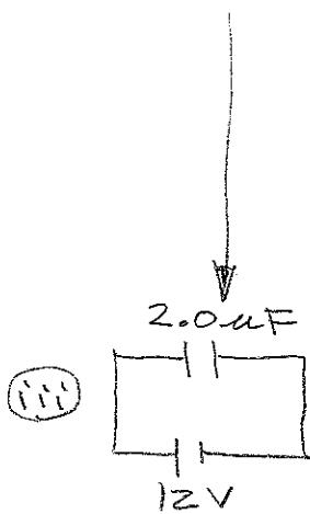
(b)  $Q = C\Delta V \rightarrow$  For case ii),  $Q = C\Delta V = (2.0 \times 10^{-6})(12V)$
