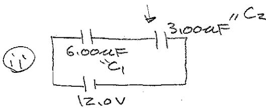
$$\begin{aligned} \frac{1}{C_{eq}} &= \frac{1}{C_1} + \frac{1}{C_2} = \frac{1}{6.00 \times 10^{-6} F} + \frac{1}{3.00 \times 10^{-6} F} \\ &= \frac{1}{10^{-6}} \left( \frac{1}{6.00 F} + \frac{2}{6.00 F} \right) \\ &= \frac{3}{6.00 \times 10^{-6} F} \\ \therefore \frac{1}{C_{eq}} &= \frac{1}{2 \times 10^{-6} F} \rightarrow C_{eq} = 2.0 \mu F \end{aligned}$$
