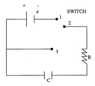
At t=0, connect 1 to 2: charge will flow from battery to capacitor plates.
