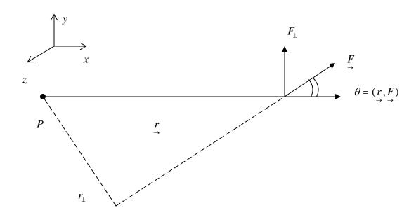
Notice that in turning the bar about an axis through P, only component of  $F \perp r$  matters or alternatively, the moment arm  $r_{\perp}$  controls  $\tau$ .
