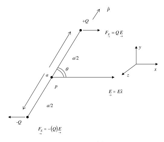
Notice there are two forces on the Dipole. +QE & -|Q|E, so total force is zero. Take torque about pivot point P (mid pt. Of Dipole). It is the sum of two torques.
