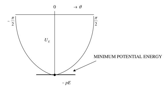
FINALLY, NOTE THAT FOR  $\, \theta << 1, U_{\scriptscriptstyle E} \alpha \, \theta^2 \, \, or \, \, \tau \, \alpha - \theta \hat{z} \,$  , so you get Linear Harmonic Oscillations, that is, for small  $\theta$  dipole will oscillate about E. In other words, dipole is in  $\equiv m$ when it is parallel to E, if you pull it aside by a small angle  $\theta$  and let go it will oscillate about E.
