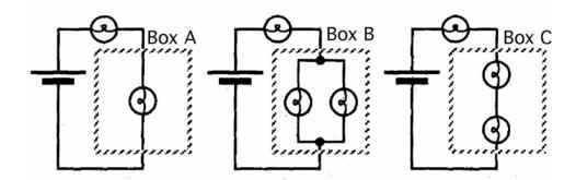
On the basis of your observations and the rule you developed at the end of the tutorial relating current through the battery to total resistance, rank the networks (boxes) A-C according to their equivalent resistance. Explain your reasoning on the basis of the model. (Do not use math.)
