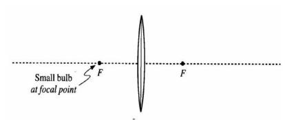
d. The light bulb is placed at one focal point of the lens as shown at right.
