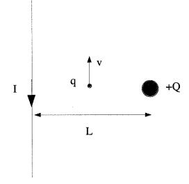
a.) (3 points) Give the magnitude and direction of the magnetic and electric fields at the location of the charge q.  $\overrightarrow{B}$  points in the  $+\widehat{z}$  direction:  $|\overrightarrow{B}| = \frac{N_0 I}{2\pi r}$  #
