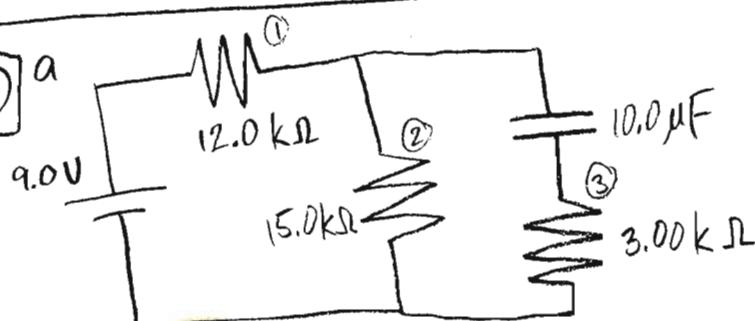
when a capacitor becomes fully charged, there is no current across it and hence no current across resistor ③ and by  $\Delta V = IR = (0)(3000) = 0$  no voltage drop also
