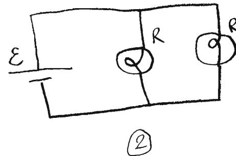
a both bulbs have the same brightness because the current is the same through both due to the symmetry of the circuit
