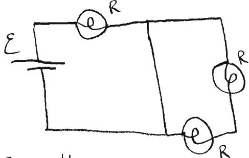
since wires are considered to have no resistance, no current flows through the branch containing bulbs ② and ③ and they are both off, hence dimmer than before
