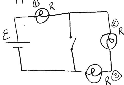
a if the switch is open, the circuit consists of three identical bulbs in series and hence all three have the same brightness
