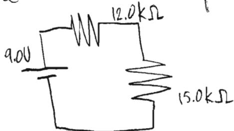
the two resistors are in series so the equivalent resistance is just  $12.0 \text{ k} + 15.0 \text{ k} = 27.0 \text{ k} \Omega$
