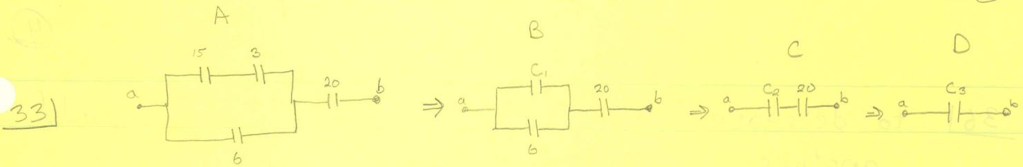
a) to find the equivalent capacitance we make the series of capacitor substitutions shown above
