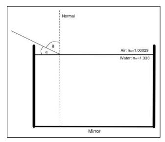
A rectangular fish tank has a bottom made with a mirror. It is filled with water (n=1.333). A laser beam is shined at an angle  $\square$ =30° from the horizontal. Consider the index of refraction of air equal to one.
