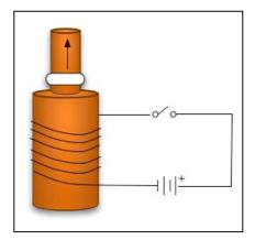
A coil is looped around a cylindrical iron core. The coil is connected to a DC generator. A metallic ring is placed around the smaller section side of the core. When the switch of the circuit is closed the ring "jumps" upward.
