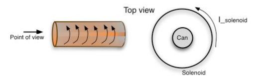
An aluminum can of radius 3 cm is inside a 100-turn and 10 cm long solenoid of wire. The electrical current inside the solenoid goes from 0 A to 100 A in a time interval of  $2\Pi 10^{-5}$  seconds.
