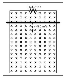
A conducting rod of mass M=0.50 Kg slides down between two vertical copper tracks at a constant speed of v=5.0 m/s perpendicular to a magnetic field B. The resistance of the rod and the tracks is negligible. The rod maintains contact with the tracks at all times and has a length L=1.5 m. A resistance R=1.75 is attached between the tops of the tracks.
