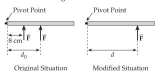
In order for the torque exerted on the door in the modified situation to equal that of the original situation, it is necessary that  $Fd = Fd_0 + F(8 \text{ cm})$  or  $d = d_0 + 8 \text{ cm}$ . Thus, the paleontologist would need to relocate about 8 cm farther from the hinge.
