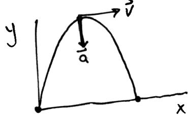
Notice  $\vec{a}$  always points down. At the peak of the path the velocity is solely in the  $x$  direction so they are perpendicular.
