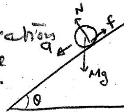
$$(3) \text{ in } (2) \quad rf = I \frac{a}{r} \quad \dots (4)$$
