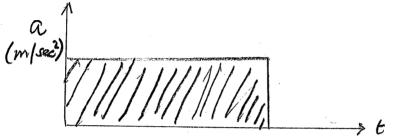
And again to write y at any time t we must know y at t = 0 and write for constant acceleration
