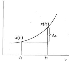
Average Velocity Vector: Measures rate of change of position with time over a finite time interval  $(t_2 - t_1)$
