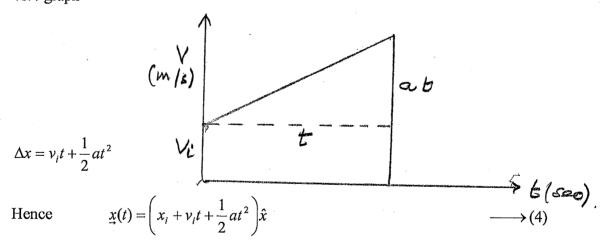
II We can use (3) to calculate average velocity between o and t since v is increasing linearly with time
