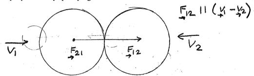
Now the forces  $\underline{F_{12}}$  and  $\underline{F_{21}}$  are parallel to the relative velocity  $(\underline{v_1} - \underline{v_2})$  so it becomes essentially a one-dimensional problem.
