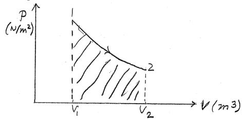
and the work done  $W_{1-2}$  is the area under the P vs. V curve.
